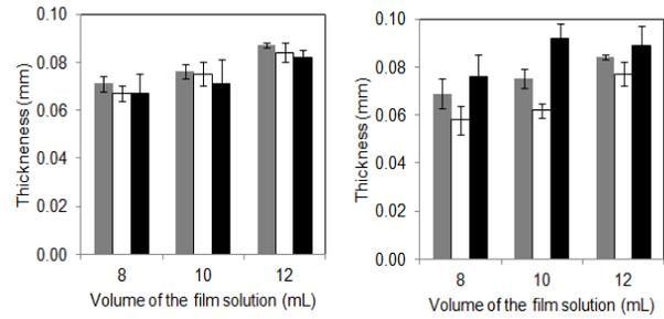
Figure 1. Film thickness of native starch and: (a) glycerol and (b) sorbitol. Gray column: Rice starch, white column: potato starch, black column: cassava starch
