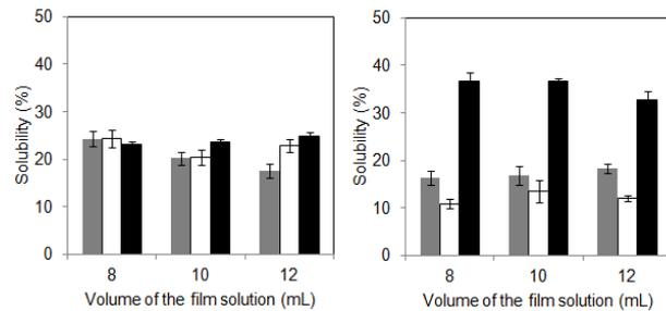
Figure 2. Solubility in water of native starch films and: (a) glycerol and (b) sorbitol. Gray column: Rice starch, white column: potato starch, black column: cassava starch
